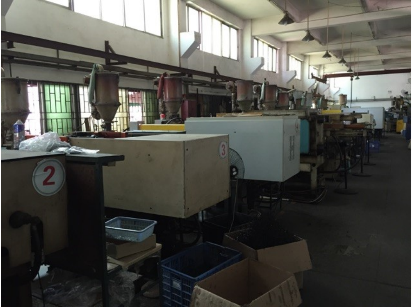
A row of plastic injection mold machines at a manufacturer of plastic parts
